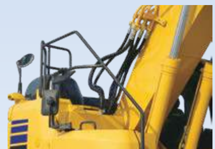
Hand rails and anti-slip plates
