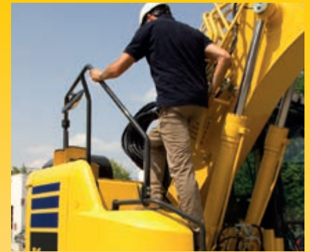
Hand rails and anti-slip plates
