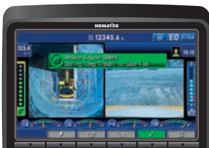
Eco-gauge, Eco guidance and fuel consumption gauge
